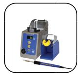
The Hakko FT802 with the FT 8003 Hot Knife is ideal for cutting and melting polyamide or polyimide tubing rated at 400 degrees celsius. This tool is nimble and can be set at different temperatures making it easy to use one tool for multiple hot knife and bonding applications.
